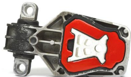
Figure 1 - showing polyurethane insert fitted inside the lower engine mount
