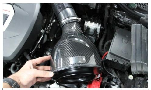
16. Push the intake into the stock plastic inlet tube – use the provided hose clamp instead of the stock spring clamp around the tube. Do not tighten yet.
