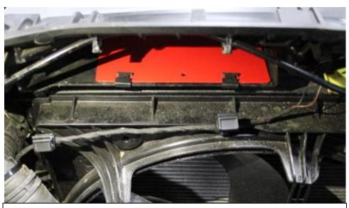
11. Push the panel clips over the scoop and the duct panel.
