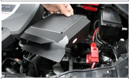
12. Take the new duct – it will be positioned in the orientation shown. Lower the duct into place.
