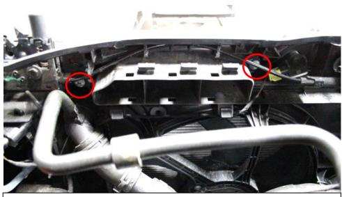
6. Remove the duct bracket by removing the 2 screws shown.
