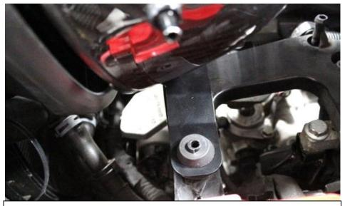
17. Lower the intake into position and push the 2 rubber mounts down into position.
