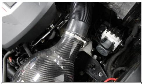
18. Now tighten the hose clamp around the tube.
