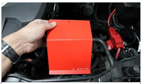
9. The scoop will go into the duct opening and will sit behind the grill in this orientation. Insert the scoop into the duct opening.
